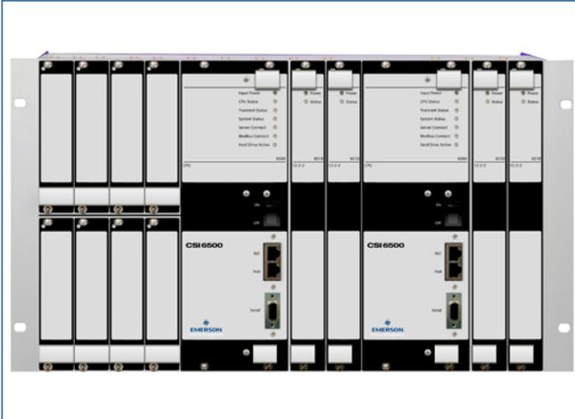
*When machinery protection already exists, or is not needed, the CSI 6500 can be deployed for machinery health monitoring. When installed in the rear signal termination configuration, the CSI 6500 can accept up to 48 vibration inputs.*
