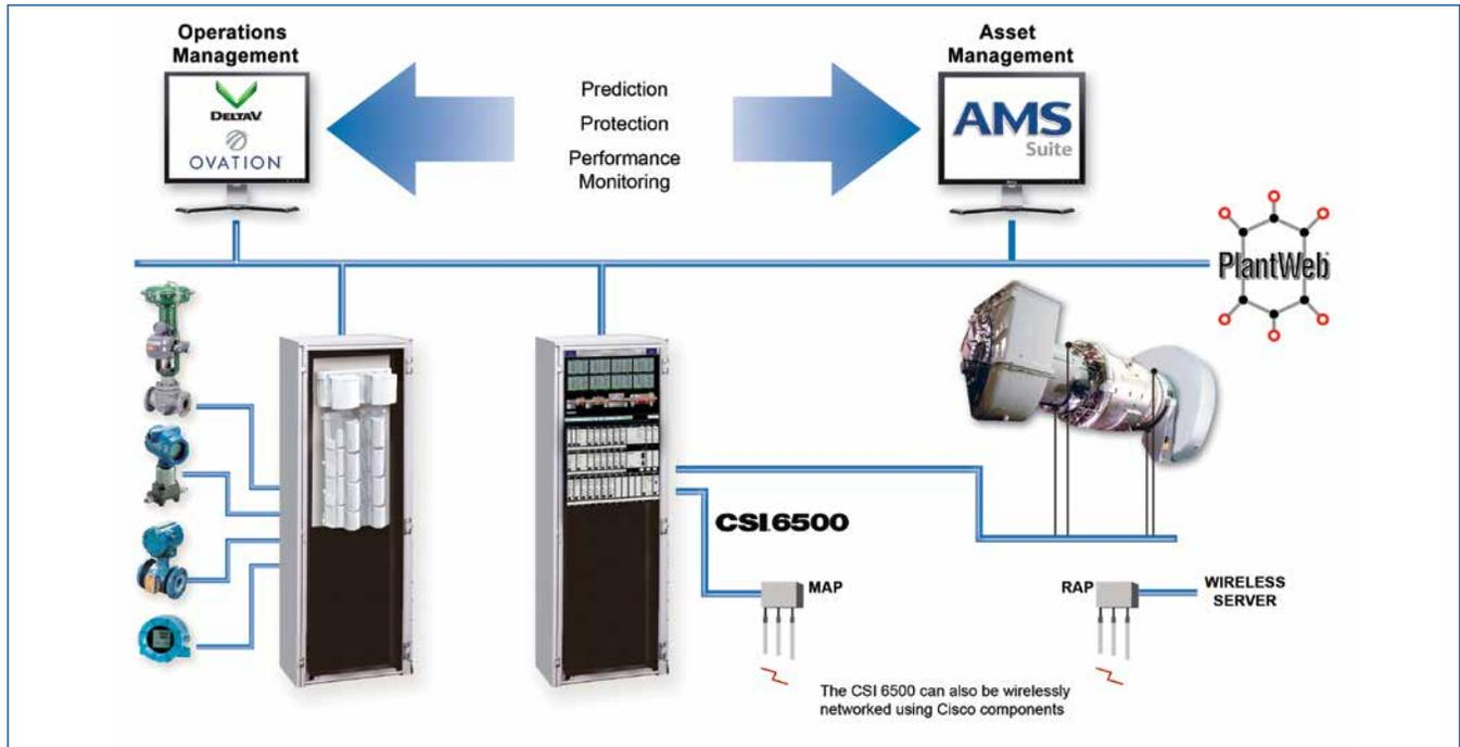
The CSI 6500 is integrated with the Ovation and DeltaV process automation systems through an easy three step process to reduce integration time from weeks to minutes. In addition, control strategies and graphical elements are automatically created, making GUI development a snap.
